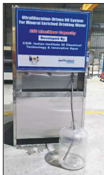
RO+UF integrated water purification system of 250L/h capacity
