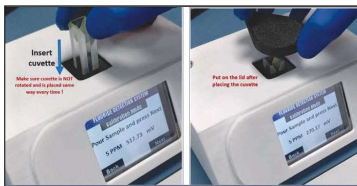
Cuvette placement and covering
