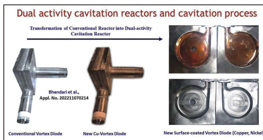
Fig 6. CSIR-NCL's Vortex Diode- Conventional and novel Surface Coated Vortex Diode
