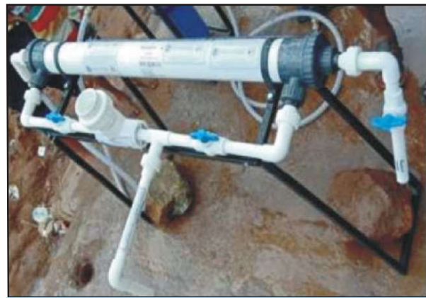
700 L/H Capacity UF System
