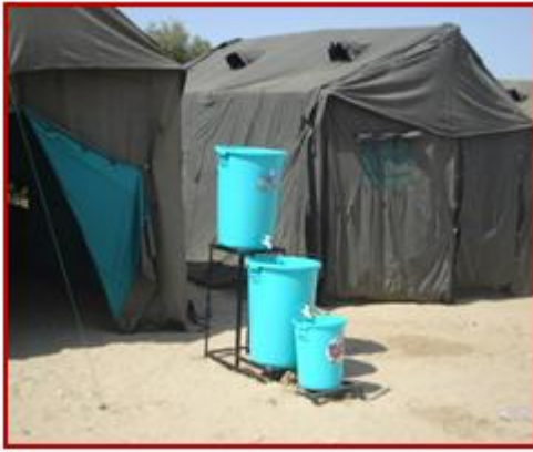
NEERI has installed 100 units in the flood affected remote areas of Barmer District in October 2006 to convert the turbid and contaminated rainwater into potable water
